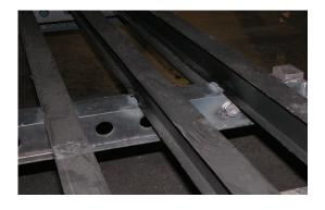
The combined strength of the Super-Sill cross members, staggered screw pattern and the solid oak flooring delivers a floor rated\* for 22,000 lbs- the best standard forklift rating in the industry. \*TTMA RP37-07
