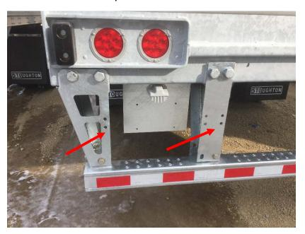
These holes are necessary for the installation of the optional steps or diagonal dock lock reinforcements. By drilling these holes on every vertical upright, we can streamline production, reduce the number of component SKUs and parts inventory, as well as reduce the number of repair parts needed by our customers. This change also makes it easier for customers to retrofit steps and dock lock reinforcements in the field.
