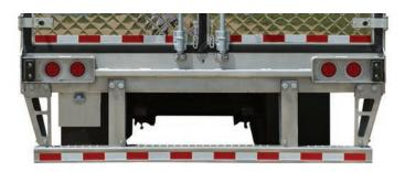
The new rear underride guard comes standard with no additional cost and weight. It resists compartmental intrusion of an automobile when the location of impact is at 30% to 100% overlap of the width of the car to the guard. It complies with all applicable U.S.and Canadian regulations. The bolt-on design allows for easy repairability.
