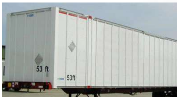
STEEL CLAD COMPOSITE PANEL
