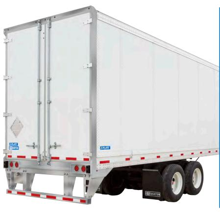
Stoughton's Z-Plate® van features include solid, full width oak floors, and extra wide extruded aluminum scuff rails and the unique recessed splice plate with "A" slots for better cargo control using any standard cargo restraint system
