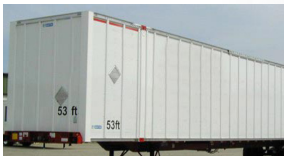
STEEL CLAD COMPOSITE PANEL
