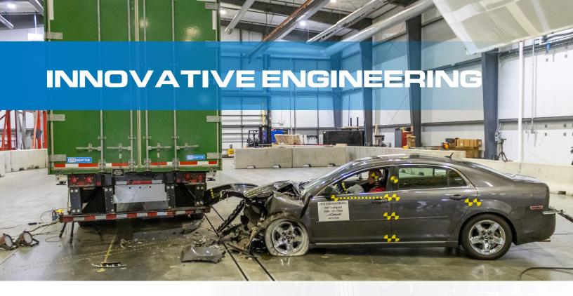
Designing an underride guard for an Intermodal Chassis presented unique challenges. Unlike dry van, refrigerated or flatbed trailers, Intermodal Chassis lack a continuous frame to support the guard. Stoughton engineers developed a new impact guard system with:
