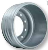
This drum has an exclusive one-piece roll-formed steel shell for superior concentricity, improved balance and reduced weight. The X30 delivers superior payload capacity and fuel economy without sacrificing strength.
