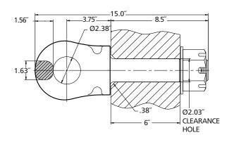
NOTE: The mounting surface must have an adequate chamfer, as shown above, so that the drawbar mounts flush with the mounting surface.
