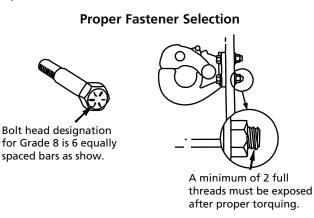
To develop the full rated capacity of a coupling device, all required mounting fasteners must be present with proper and equal torque applied to each fastener. Torque values and procedures should follow SAE J429 and are stated in the Owner's Manual shipped with each Holland coupling product. This information is also available online at the SAF-HOLLAND website.
