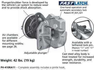
PH-410RA11 – Complete assembly includes a pintle hook, plunger, air chamber, and mounting bracket.
