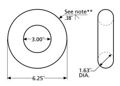
\*\*NOTE: 8.5<sup>°</sup> of linear weld .38<sup>°</sup> bevel groove weld (3<sup>°</sup>x 1.25<sup>°</sup> bar used) required to obtain ratings.
