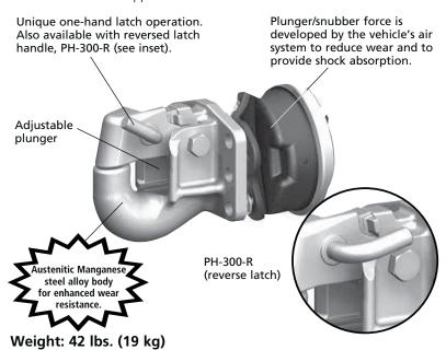
The complete assembly includes a pintle hook, plunger, air chamber, and mounting bracket. For pintle hooks without an air chamber, bracket, or plunger, order PH-300-1 or PH-300-R-1.
