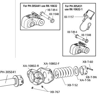
Available with a tethered lock pin as PH-30SE51.
