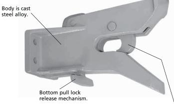
Jaw remains open upon lock release and automatically closes and locks when drawbar is inserted.
