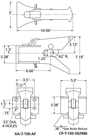
**NOTE:** Maximum of 16.76 linear inches of .38" fillet weld required to develop rated capacity.
