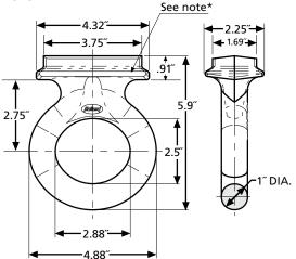
\*NOTE: A minimum of 12<sup>"</sup> linear inches of .38<sup>"</sup> weld on 2<sup>"</sup>x 4<sup>"</sup> (11 gauge) structural tubing required to obtain ratings.
