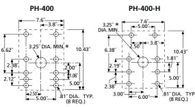
\* Center hole not required if used without air chamber.
