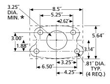
\* Center hole not required if used without air chamber.
