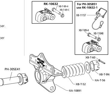
Available with a tethered lock pin as PH-30SE51.
