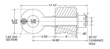
NOTE: The mounting surface must have an adequate chamfer, as shown above, so that the drawbar mounts flush with the mounting surface.
