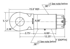
**\*NOTE:** Minimum of 24 linear inches of .38<sup>"</sup> fillet weld required to develop rated capacity.
