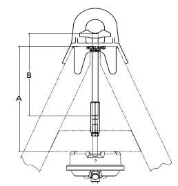
**A** = Distance required to mount air chamber **B** = Rod length
