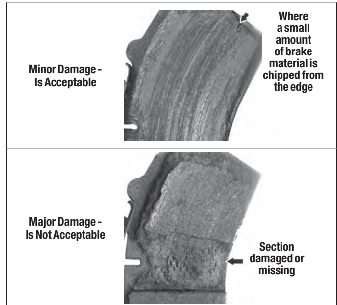
Figure 24 – Brake Pad Surface Inspection
