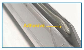
Apply a 3/16" diameter bead of Sea-Lok adhesive sealant at mid point on each inside wall of rigid channel. Using the same adhesive sealant, apply beads to corner fiber tab. Note: complete next step within 10 minutes of sealant application.
