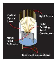
Because filament failure is not a concern for LED lights, they have an extremely fast turn-on time, and can last up to 100,000 hours. Combine this with their durability, and it's clear that they are ideal for the heavy duty industry.
