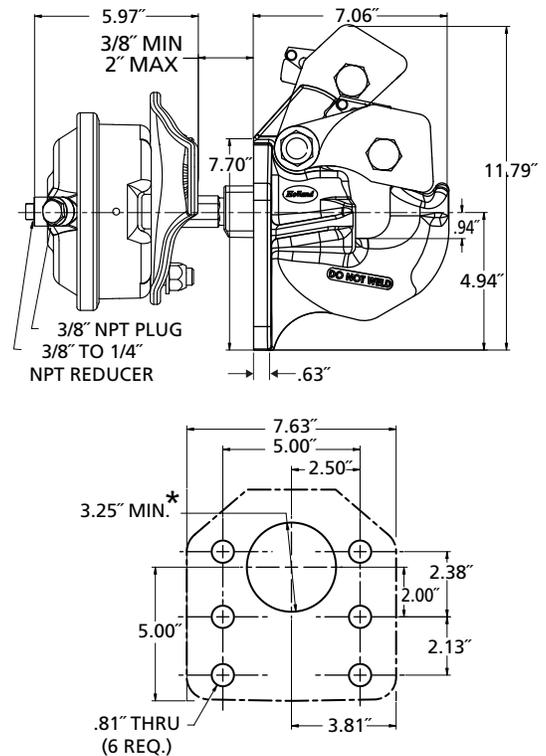
\* Center hole not required if used without air chamber.
