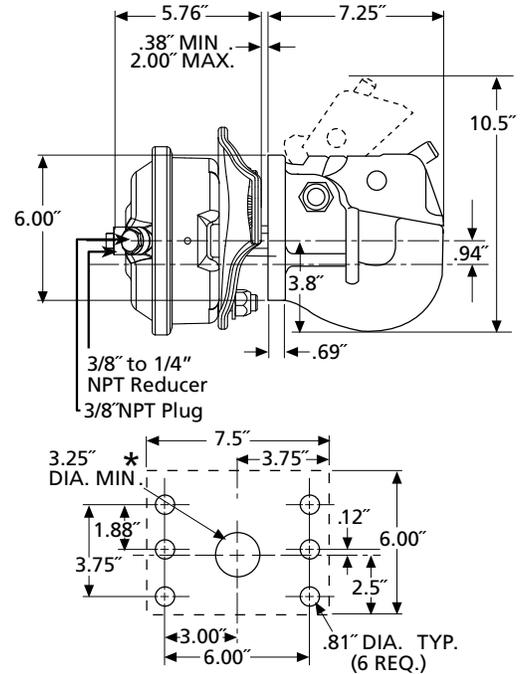
\* Center hole not required if used without air chamber.
