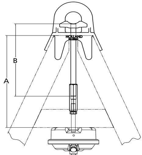
**A** = Distance required to mount air chamber
