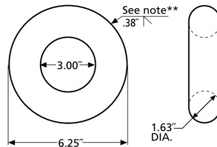
\*NOTE: A minimum of 12" linear inches of .38" weld on 2"x 4" (11 gauge) structural tubing required to obtain ratings.
