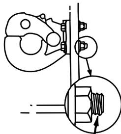
A minimum of 2 full threads must be exposed after proper torquing.
