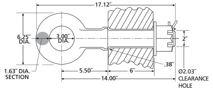
**\*NOTE:** Minimum of 24 linear inches of .38" fillet weld required to develop rated capacity.
