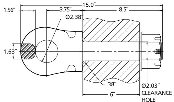
**\*NOTE:** Minimum of 24 linear inches of .38" fillet weld required to develop rated capacity.
