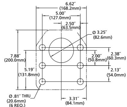
\* Center hole not required if used without air chamber.
