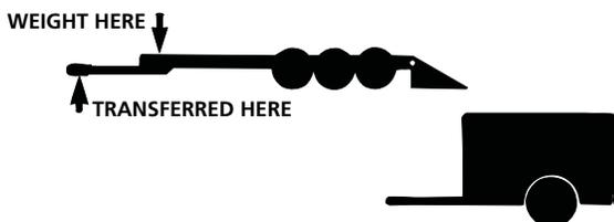
The type of load, density of the load, and placement of the load in relation to the trailer axles will have a significant effect on the vertical load at the trailer tongue. Excessive vertical loads, approaching 20% of gross trailer weight, can result in accelerated wear and over-loading of the coupling devices.
