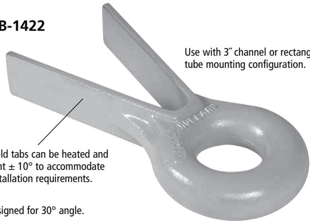
Weld tabs can be heated and bent  $\pm 10^\circ$  to accommodate installation requirements.
