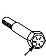
Bolt head designation for Grade 8 is 6 equally spaced bars as show.
