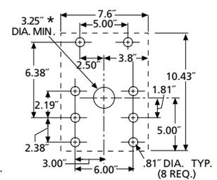
\* Center hole not required if used without air chamber.
