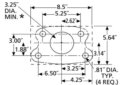
\* Center hole not required if used without air chamber.
