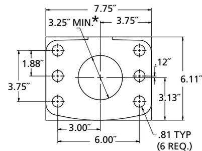
\* Center hole not required if used without air chamber.
