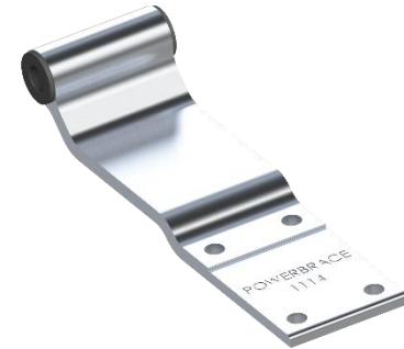
P11144 Glide-Pro Hinge with Bearings 9-1/2" Long, 2-3/4" Wide, 4 Hole, 1-5/8" Offset Used with: 2-3/4" Hinge Butts Extra-Long offset for wide door posts
