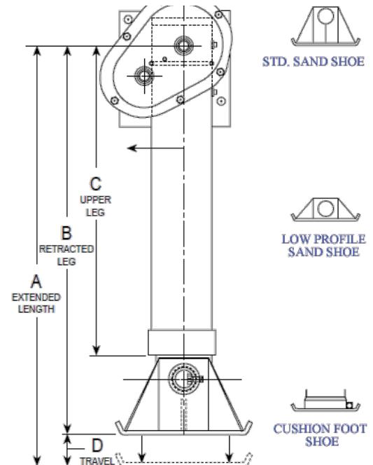
**Common Industry Terms** Prop legs, Support legs, Dolly legs, Gear-side (Drive leg), Non-Gear Side (Slave leg)
